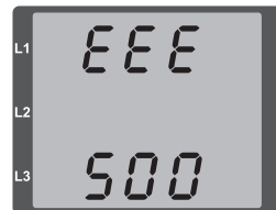
Fig. Warning message with number 500 (mains frequency)
