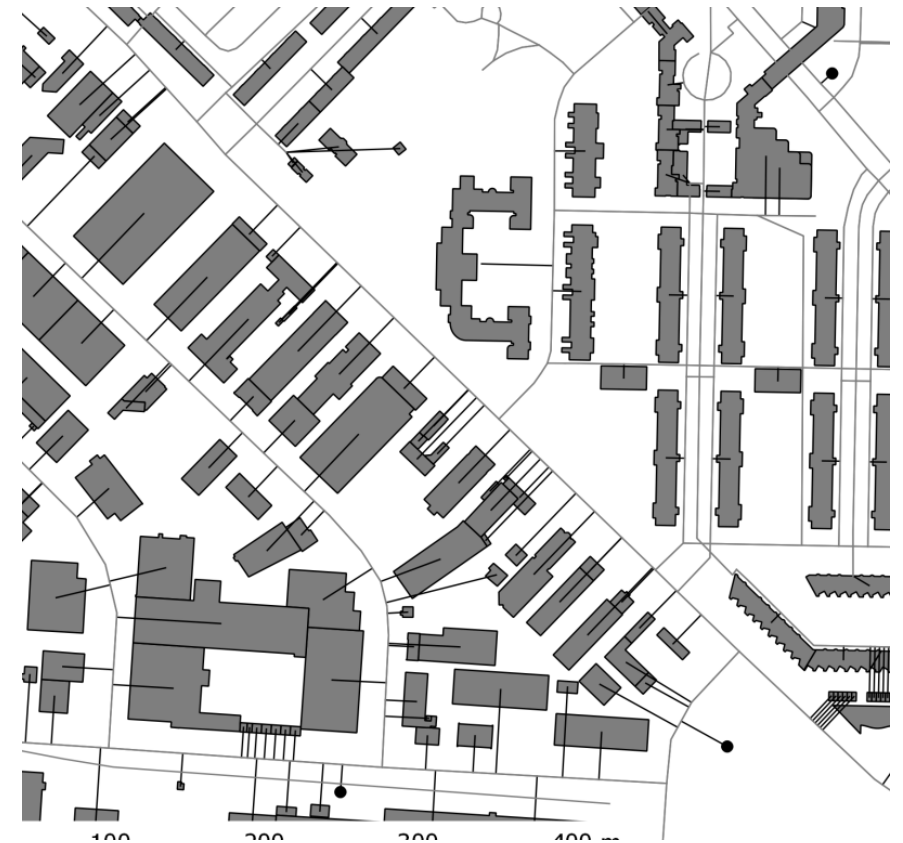
Figure 4: Attaching sources/sinks to the road network
